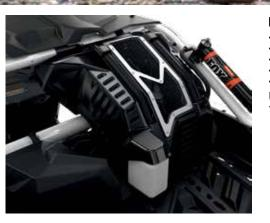
New SNORKEL PRE-FILTER · Pre-filter specifically for snorkels. · Adds extra protection to your engine in harsh riding conditions. · Helps keep air filter cleaner.
