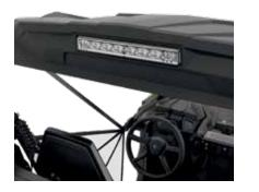
DOME LIGHT · LED array integrates perfectly with vehicle. ·Wiring included. ·Can be installed on cage, Sport Roof or All-Terrain Trunk Cover Maverick Trail, Maverick Sport, Maverick Sport MAX 715002455
