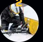
Drive straight toward the plow. Attach the winch cable to the plow using a guiding hook/roller.
