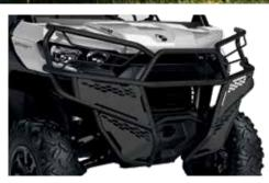
Defender, Defender MAX (2020) · Improved approach angle. · Compatible with front rack, snow plows, tire and track kits, winches. 715005410
